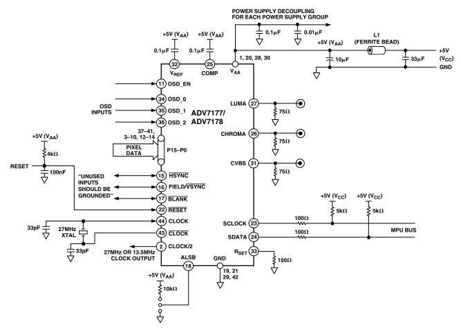
Figure 43. Recommended Analog Circuit Layout
