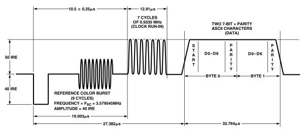
Figure 44. Closed Captioning Waveform (NTSC)
