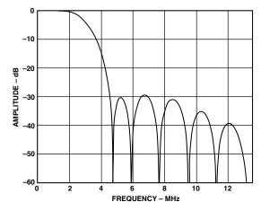
Figure 10. PAL Notch Filter
