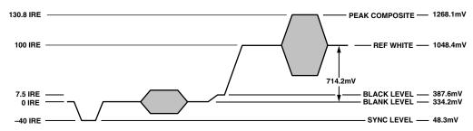
Figure 45. NTSC Composite Video Levels
