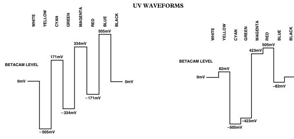
Figure 57. NTSC 100% Color Bars No Pedestal U Levels
