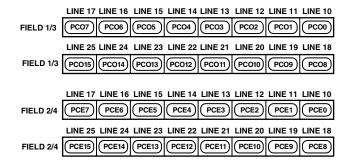
Figure 40. Pedestal Control Registers
