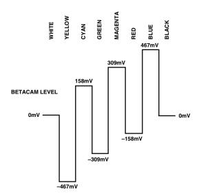
Figure 58. NTSC 100% Color Bars with Pedestal U Levels
