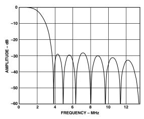
Figure 8. NTSC Notch Filter
