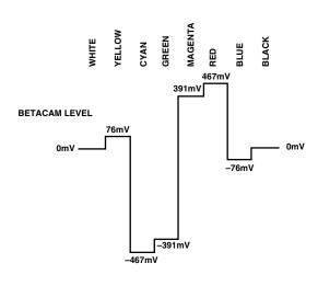
Figure 61. NTSC 100% Color Bars with Pedestal V Levels
