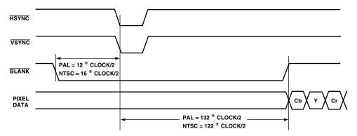
Figure 23. Timing Mode 2 Even-to-Odd Field Transition Master/Slave
