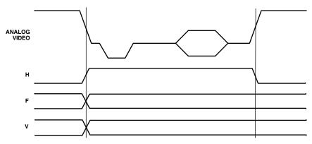
Figure 17. Timing Mode 0 Data Transitions (Master Mode)
