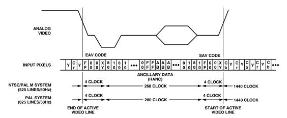
Figure 14. Timing Mode 0 (Slave Mode)
