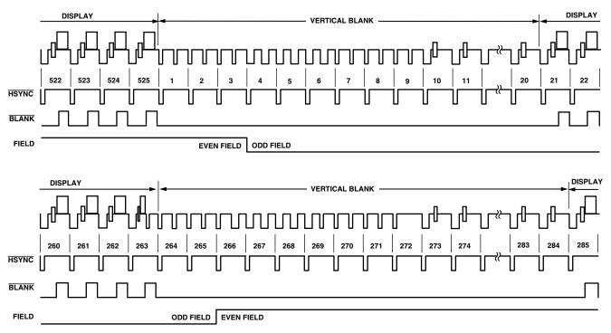
Figure 18. Timing Mode 1 (NTSC)
