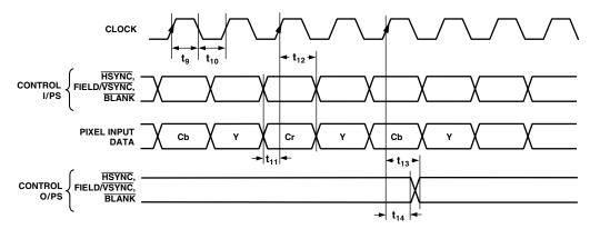
Figure 2. Pixel and Control Data Timing Diagram
