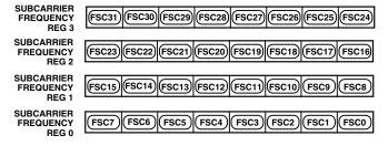
Figure 34. Subcarrier Frequency Register
