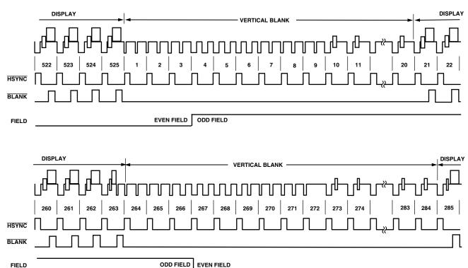
Figure 25. Timing Mode 3 (NTSC)
