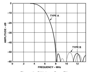
Figure 9. PAL Low-Pass Filter
