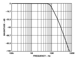
Figure 64. Output Filter Plot
