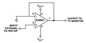
Figure 68. Recommended Output DAC Buffer
