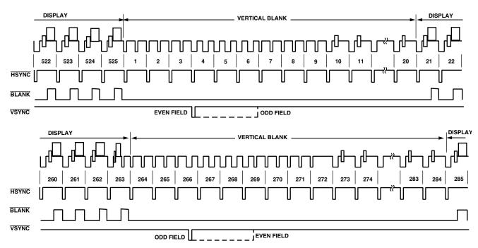
Figure 21. Timing Mode 2 (NTSC)
