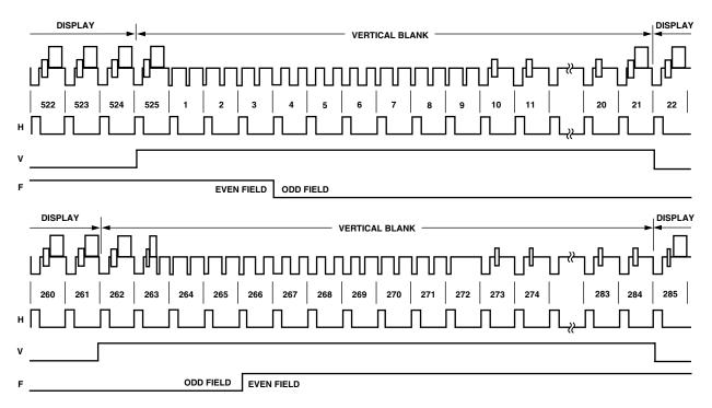
Figure 15. Timing Mode 0 (NTSC Master Mode)
