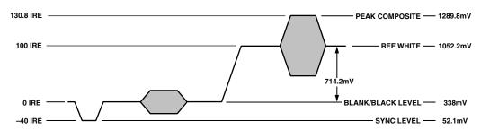
Figure 49. NTSC Composite Video Levels
